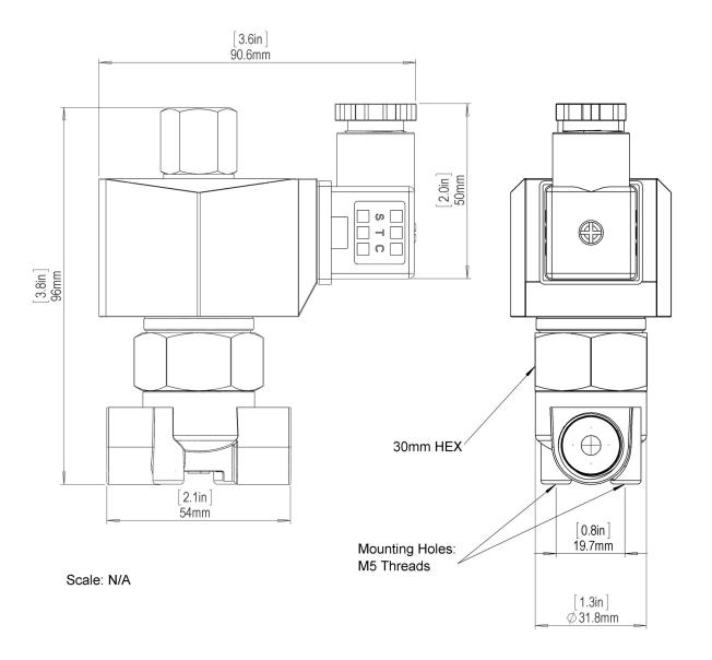
Note: Dimensions are for reference only. Field verify dimensions prior to installation for critical dimensions.
