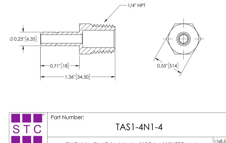
316 Stainless Steel Tube Adaptor, 1/4" Tube, 1/4" NPT Thread
